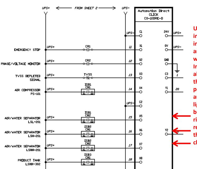
Usually an open input has no indication light and a closed input will have a light. In this example if all the floats are in the resting position then X5 an X6 will have no light and X7 will be lit. If a float rises from its resting position the lights will change status.
