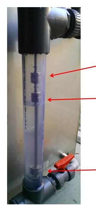
Looking at the floats, the water level has caused the Low float to rise but has not reached the High float or the High High float which are still in their resting positions
