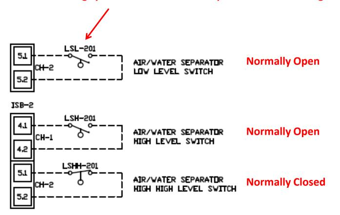
Look at the electrical drawings to find out what inputs turn on and off when the floats change position. The Air Water Separator floats are connected to X5, X6 and X7 as shown below.
